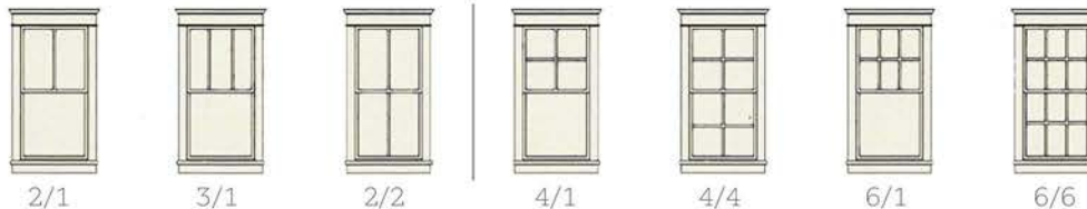
WINDOWS - Heavier head trim detail is suggested
